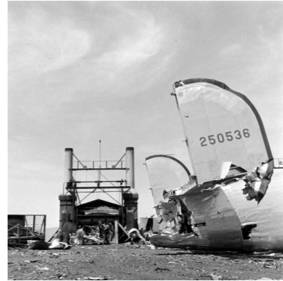
2. The pieces are moved to the smelter in the distance while Ford-built B-24J 42-50536 waits its turn
